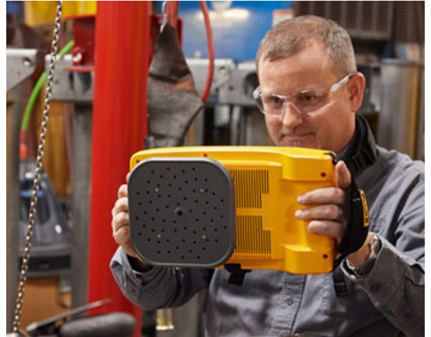
Figure 4: Detecting leaks using the full array microphones.
