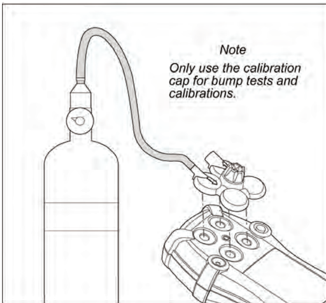
Figure 11. Connecting the Gas Cylinder to the Detector
